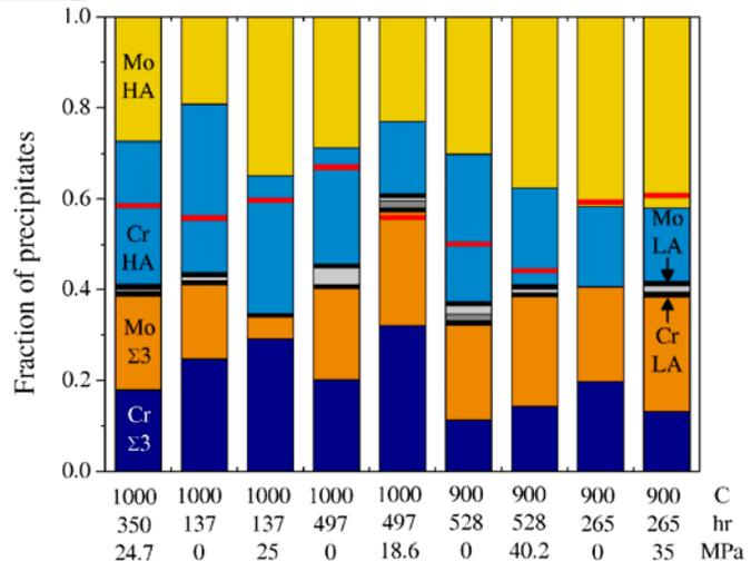
Figure 3: Distribution of grain boundary precipitates by boundary and precipitate type. The red line shows the overall fraction of  $\Sigma 3$  + low-angle boundaries in the specimen. Each column represents a different test condition.
