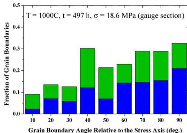
Figure 4: Fraction of grain boundaries populated by precipitates as a function of the angle between the grain boundary trace and applied stress axis for the grip (left,  $\sigma \sim 0$ ) and gauge (right,  $\sigma > 0$ ) for the specimen tested at 1000°C and 18.6 MPa.
