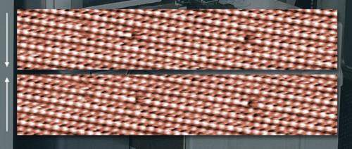
Successive AC mode topography images of the cleavage plane of a calcite crystal in water. The repeated point defects demonstrate the true atomic resolution capabilities of the Cypher AFM. Arrows indicate scan direction. Scan size 20nm; Z scale 3.2Å; Cantilever Amplitude 4Å; Cantilever Frequency 454 kHz.
