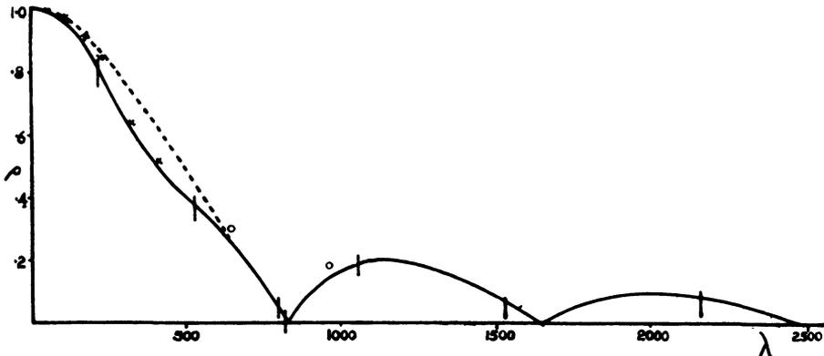
FIG. 1. Cassiopeia A, amplitude of the visibility function at 127 Mc/s in position angle  $90^\circ$ . The vertical lines represent the readings taken in 1956 with the phase sensitive interferometer. The circles are readings by Jennison and Das Gupta and the crosses are readings by Smith.
