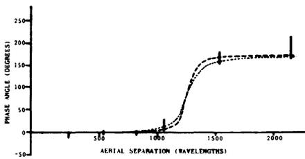
FIG. 6. Cygnus A, phase of the visibility function at 127 Mc/s, in position angle 90°. The vertical lines refer to the observed readings whilst the two curves correspond to the two distributions in Fig. 7.
