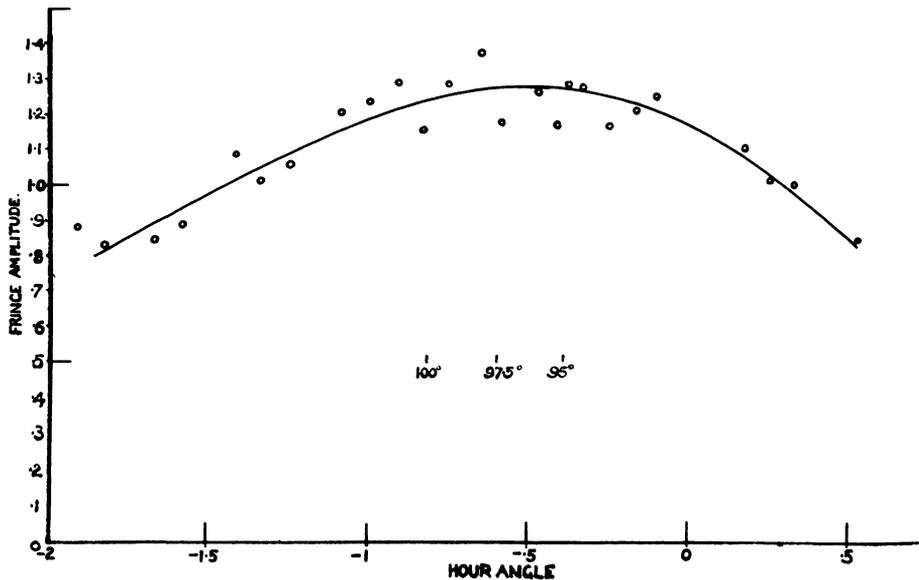
FIG. 8. Cygnus A, 127 Mc/s. Variation of fringe visibility with position of source for the determination of the position angle of the major axis. Azimuth of the baseline of the interferometer  $177^\circ$ . The scale in the center of the diagram gives the position angle corresponding to the maximum fringe visibility.
