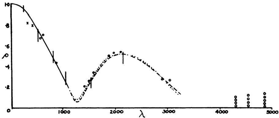
FIG. 5. Cygnus A, amplitude of visibility function at 127 Mc/s in position angle 90°. The vertical lines represent readings taken with the phase sensitive interferometer. The crosses are readings by Smith and the circles are readings by Jennison and Das Gupta, the readings between 4000 and 5000 wavelengths were zero in the latter measurements of the function  $\rho^2$ , on conversion to  $\rho$  the errors are as shown. The two curves refer to the alternative brightness distributions in Fig. 7.
