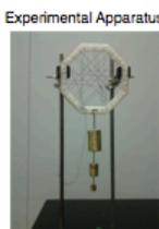
Students wove the experimental and control webs using commercially available cotton sewing thread as an analogue for the spider silk. Looms were suspended vertically and laboratory weights were added to the unattached side of the octagon until the web failed
