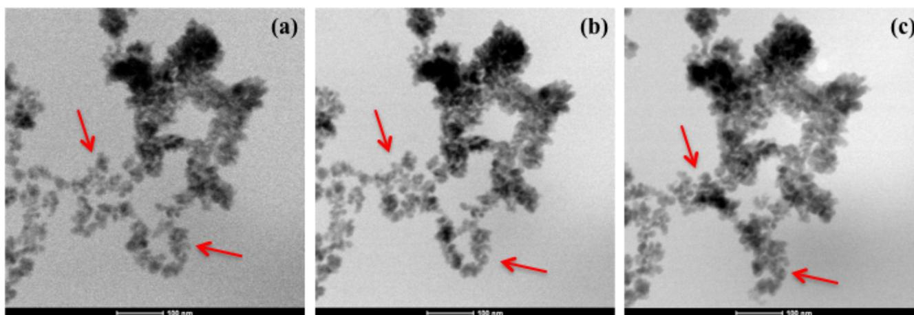
Figure 1. *In situ* STEM-BF images showing the further development of asphaltene coalescence of an agglomerate after 4 h in the oil + heptane emulsion (a) and after 1 min (b) and 3 min (c) under the electron beam. The aggregation process is driven by the agglomeration of 10-20 nm asphaltene clusters (marked by red arrows).
