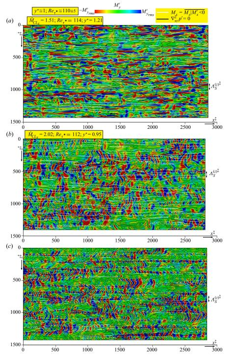
Figure 17. Instantaneous wall-normal Mach number fluctuation  $M'_y$  (colourmap  $-M'_{y_{rms}} \leq M'_y \leq +M'_{y_{rms}}$ ), on  $(x^{\ddagger}, z^{\ddagger})$  planes very near the wall  $(y^{\star} \approx 1)$ , for different  $\overline{M}_{CL_x} \in \{1.51, 2.02, 2.49\}$  at nearly constant  $Re_{\tau^{\star}} \approx 110$ ; also included are approximate streak boundaries (white contours  $M_x = \overline{M}_x|_{M'_x < 0}$ ) and p'-fronts (black contours  $\nabla_{xz}p' = 0$ ).
