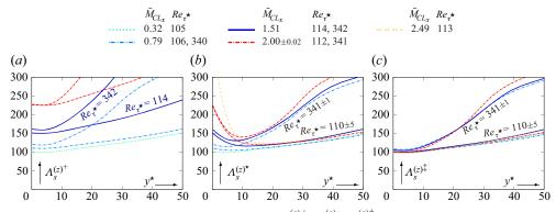
Figure 11. Different non-dimensionalisations (2.1)  $\{\Lambda_S^{(z)+}, \Lambda_S^{(z)+}, \Lambda_S^{(z)+}, \Lambda_S^{(z)+}\}$  of the surrogate for the average spanwise distance (4.2*b*), (4.2*c*), plotted against the HCB-scaled non-dimensional distance from the wall  $y^*$  (2.1*b*), at nearly constant  $Re_{\tau^*} \in \{110\pm 5, 341\pm 1\}$  for different  $\overline{M}_{CL_x} \in \{0.32, 0.79, 1.51, 2.00\pm 0.02, 2.49\}$  (table 2); enlarged view of the region  $y^* \leq 50$ .
