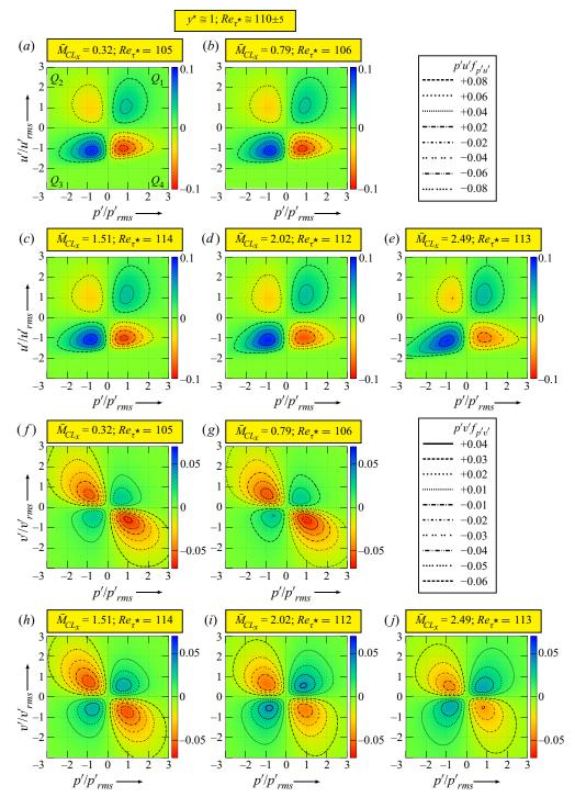
Figure 16. Integrands in the calculation of the correlation coefficients  $c_{p'u'}$  (4.5*a*) and  $c_{p'v'}$  (4.5*b*) from the corresponding joint p.d.f.s, plotted against the standardised variables  $\{p'/p'_{rms}, u'/u'_{rms}, v'/v'_{rms}\}$ , very near the wall ( $y^* \approx 1$ ), at nearly constant  $Re_{\tau^*} \approx 110$  for different  $\bar{M}_{CL_x} \in \{0.32, 0.79, 1.51, 2.02, 2.49\}$ .
