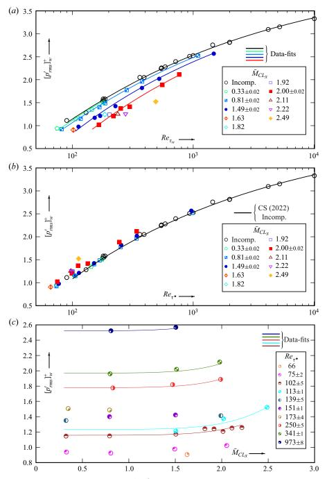
Pressure fluctuations in compressible wall turbulence
