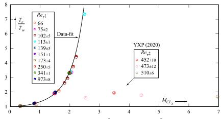
Figure 6. Variation of wall-cooling ratio  $1 < T_r/\bar{T}_w \lesssim 7.35$  (0.136  $\lesssim \bar{T}_w/T_r < 1$ ) and centreline Mach number  $0.32 \lesssim \bar{M}_{CL_x} \lesssim 6.97$  for the present data (table 1) and for the Yu *et al.* (2019, 2020) DNS data (YXP, 2020), for varying  $66 \leqslant Re_{\tau^{\ddagger}} \leqslant 983$ .
