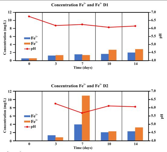
Fig. 11 Fe<sup>2+</sup> and Fe<sup>3+</sup> concentrations (mg/L) and pH during the bioleaching experiments with the *Bacillus* strain
