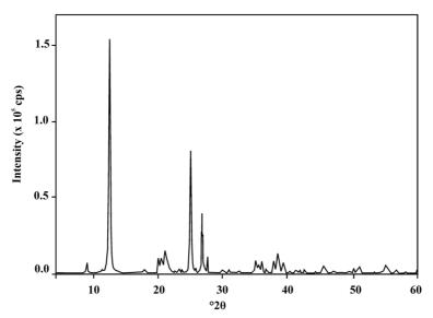
Fig. 1 XRD of high-iron kaolin
