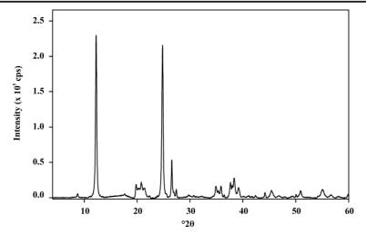
Fig. 2 XRD of kaolin sample from RSM 4 experiment
