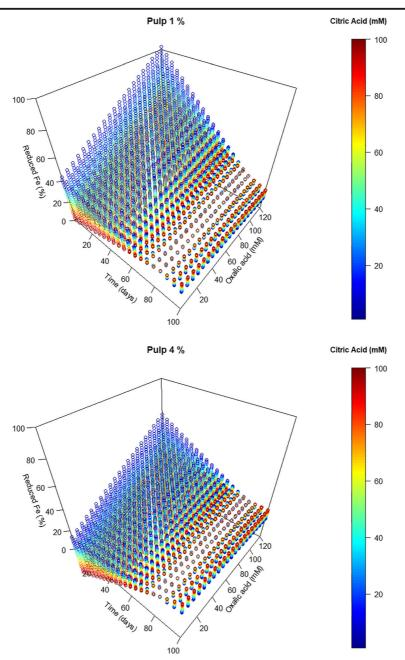
**Fig. 4** Response Surface Methodology (RMS) curves for 1, 4, and 7% pulp concentrations. The *z*-axis represents the Fe reduction (%) after Eq. 1; the *y*-axis represents the oxalic acid concentration (mM); and the *x*-axis represents the time (days)
