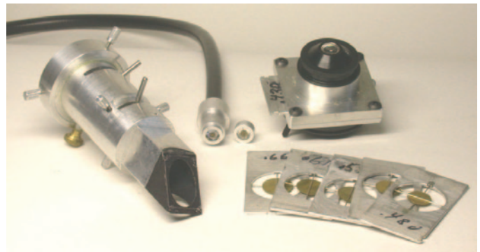
Figure 3: Reflected light illuminator (left) with the modified aplanatic condenser lens and COL stops (right).
