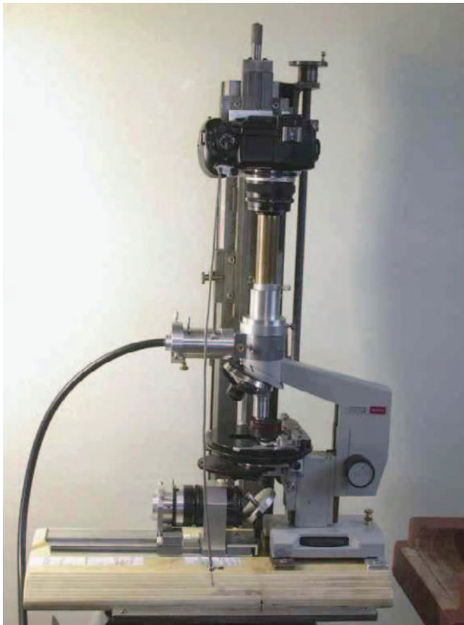
Figure 1: Modified Biolam microscope equipped with a reflected light (epi) illuminator capable of COL. Olympus E-330 DSLR camera with a 28 mm f/2.8 wide angle lens focused at infinity is separately mounted to the stand over the eyepiece.
