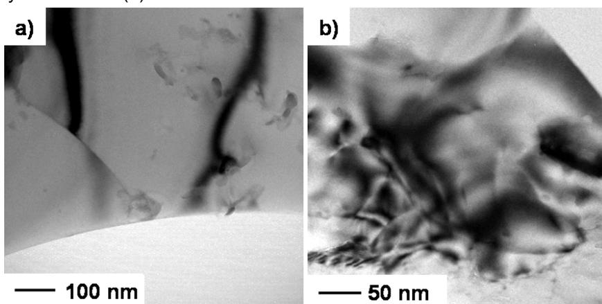
**Figure 2.-** TEM bright field image of an Al-based composite. Additional to the bend contours and grain boundaries in (a) note that there is a continuous distribution of dark spots which correspond to Fe particles, better observed in (b).
