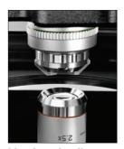
This new microscope combines light sheet microscopy and confocal microscopy in one system without compromising either functionality. It allows the combination of the two methods, for example, confocal photomanipulation with subsequent light sheet acquisition. Light sheet fluorescent microscopy (LSFM) reduces phototoxic effects and fluorophore
