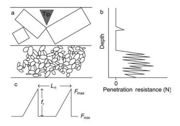
**Fig. 2.** (a) Schematic of poorly bonded (top) and well-bonded (bottom) snow layers and (b) the corresponding schematic SMP signals. (c) Definition of the microstructural parameters, rupture force,  $f_{rr}$  element length,  $L_{nr}$  and peak force,  $F_{maxr}$  and the corresponding minimum,  $F_{min}$ . The number of peaks,  $n_{peaksr}$  corresponds to the number of ruptures per unit length.
