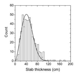
Fig. 3. Frequency distribution of slab thickness from 512 stability tests performed in the Swiss Alps and the Columbia Mountains of western Canada, and the fitted Weibull distribution (solid curve).
