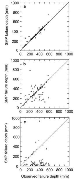
**Fig. 5.** (a) Failure depth derived from rutschblock test and compression tests vs failure depth selected manually from the four suggested weak layers (accuracy 90%). (b) Comparison of the observed failure depth to the failure depth of the weak layer derived with Equation (5) (accuracy 60%). (c) Comparison of the position of the lowest measured penetration resistance to the observed failure depth (accuracy 10%). The solid line in each graph shows the one-to-one relationship.
