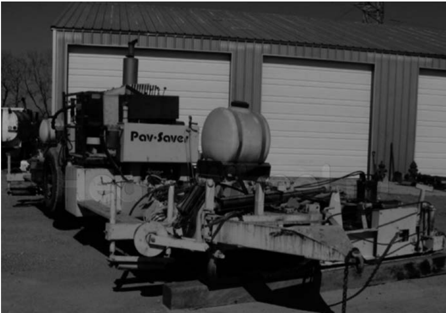
FIGURE 9.4 A Pav-Saver road-paving machine.
