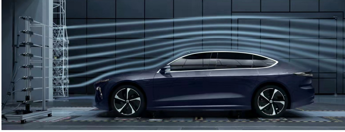
Figure 2.9 Streaklines used to visualize subsets of streamlines in a steady flow around a Nio ET7 electric vehicle. Image: Courtesy of Nio Inc.
