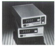
Digital Thermometers: Single-channel and eight-channel digital thermometers with SOFTCAL software can be coupled with DT-470 diode sensors for operation from -272°C to 202°C. System accuracy is ±0.5°C or better from -243°C to 100°C and within 0.1°C in an 80°C band around the calibration point. Thermometers can scan multiple sensors, monitor alarm points, and transmit to a printer. Lake Shore Cryotronics, 64 East Walnut Street, Westerville, OH 43081; (614) 891-2243.
