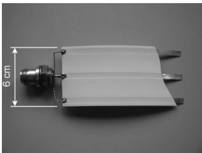
Fig. 1. The insulated flat-band cable (short section with uncovered conductor to show connection and geometry).
