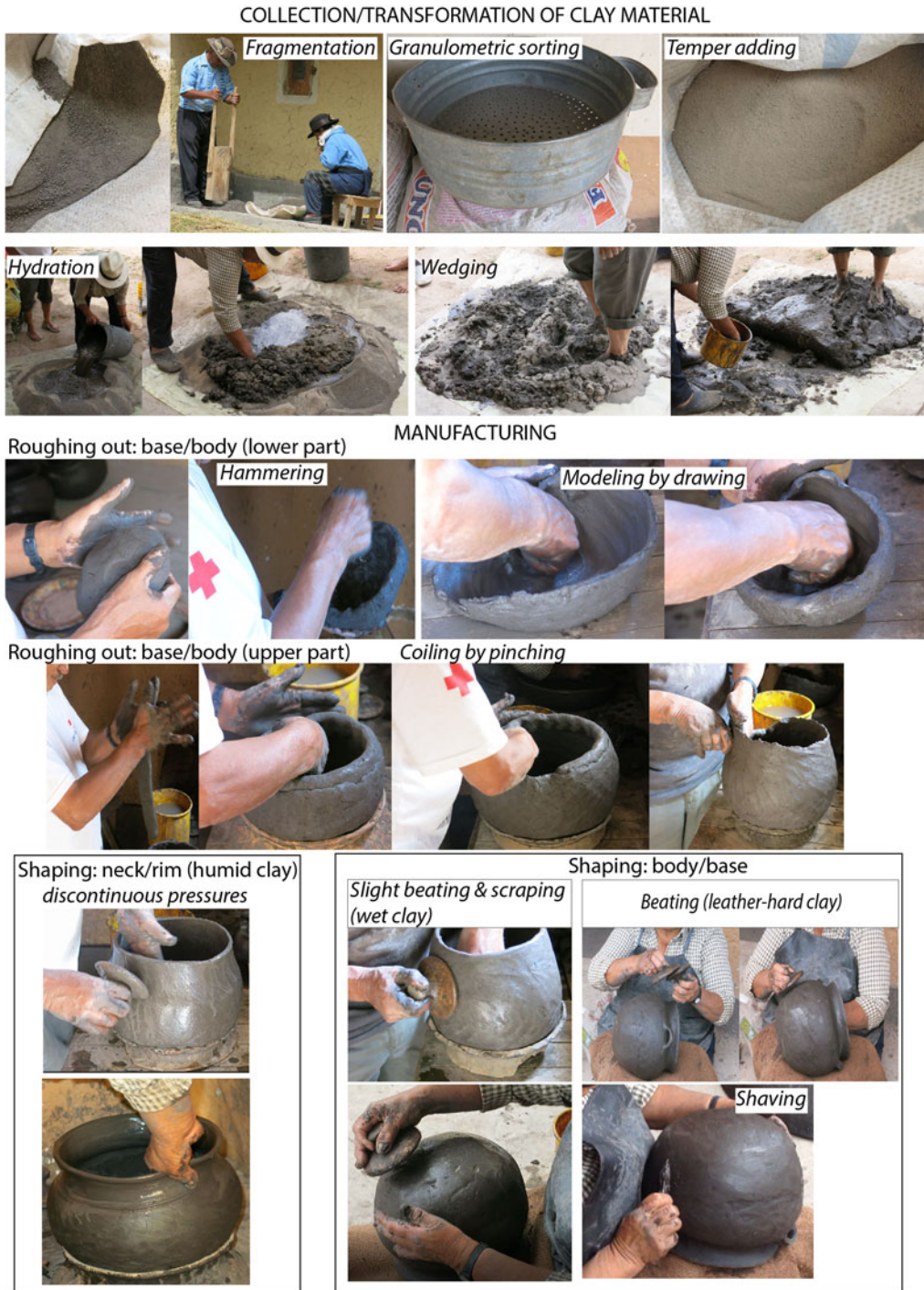
Figure 3. Pottery chaîne opératoire in Nabon: collection/transformation of clay material and manufacturing (photos by Catherine Lara). (Color online)
