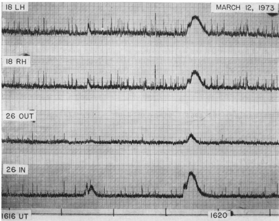
Fig. 3. Unresolved solar millisecond pulses at 18 and 26 MHz. Some of the pulses recorded on the 26 MHz in-phase channel do not appear simultaneously on the other three channels.
