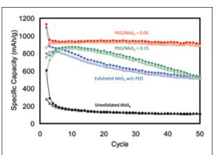
Comparison of cycling stability for unexfoliated MoS<sub>2</sub> and exfoliated MoS2 with different amounts of polyethylene oxide (PEO). All cells were cycled between 0.01 V and 3.0 V at 50 mA/g. Solid symbols, Li insertion; open symbols, Li extraction. Reproduced with permission from Chem. Mater. 22 (16) (2010) DOI:10.1021/cm101254j; p. 4522. © 2010 American Chemical Society.
