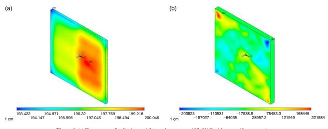
Figure 6. (a) Temperature distribution and (b) xy shear stress of Yb:YAG with non-uniform pumping.
