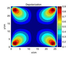
Figure 4. Depolarization of one Md:glass disk.
