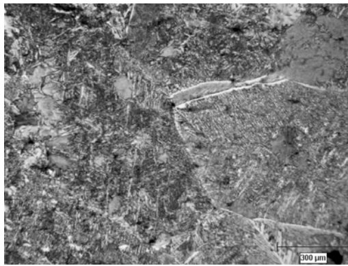
FIG. 5. Quenched sample of plain carbon steel revealing proeutectoid ferrite along the grain boundaries at minimum ductility.
