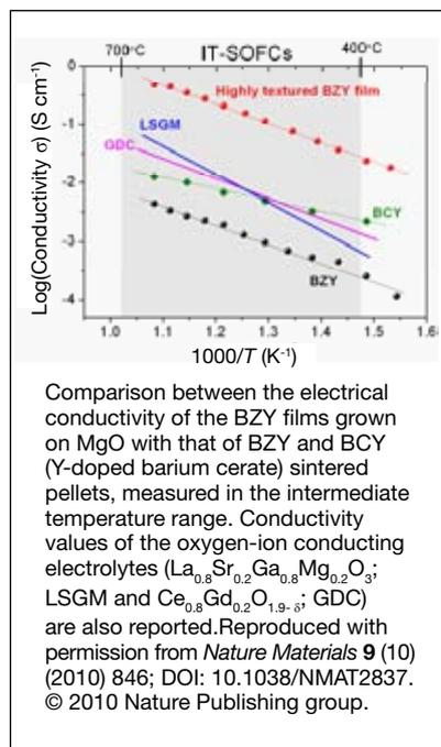
cells, at a temperature as low as 350°C (see figure). As seen in the figure, BZY film conductivity is significantly larger than best performing, stable oxygen-ion conductors used for SOFC applications in the intermediate temperature range. The researchers carried out an extensive in-plane x-ray diffraction analysis to confirm the crystalline nature of epitaxially grown BZY films and to obtain reciprocal space maps.
