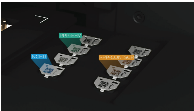
Figure 8: The QR code reader identifies the probe type by reading the QR codes on the chip carriers in the probe cassette.
