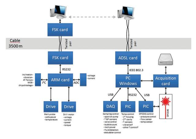
Fig. 6. Schematic of the date transmission lines.
