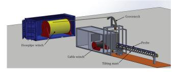
Fig. 10. Schematic of surface equipment.
