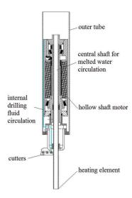
Fig. 3. Schematic of the lower part of the probe (drill head and motor section).
