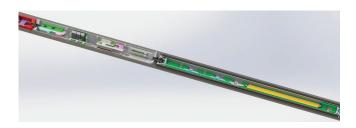
**Fig. 5.** Schematic of the OF-CEAS spectrometer with its thermal regulation shield.
