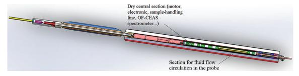
Fig. 2. Internal fluid circulation in the probe.
