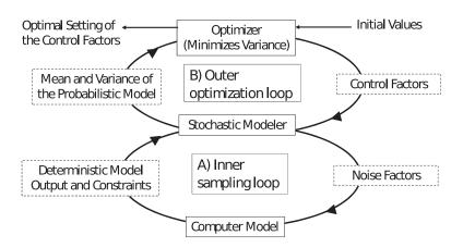
**Figure 1.** Schematic description of robust design including a sampling loop embedded within an optimization loop (Adapted from Kalagnanam & Diwekar 1997).
