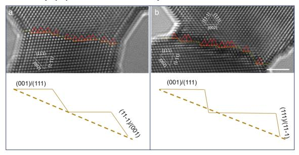
**Figure 1.** HRTEM images and schematic illustrations showing the two types of faceted asymmetrical GB in the fabricated bicrystals. (a) Type 1 GB consisting of (002)/(111) + (-1-11)/(002) facets, (b) type 2 GB consisting of (002)/(111) + (111)/(11-1) facets. Scale bar, 2nm.
