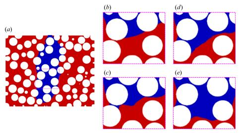
Figure 10. Liquid distribution on the YZ plane at  $X = 1.5 d_p$  at (a) breakthrough and enlarged view of the liquid distribution on the cut portion (marked by purple dashed lines) at  $t/t^*$  of (b) 0.53, (c) 0.59, (d) 0.65 and (e) 0.71 displaying the time evolution unified void filling event. Note: liquid and gas are coloured blue and red, respectively;  $AB_s = 1.83 \times 10^{-1}$ ,  $We_s = 6.18 \times 10^{-3}$ .
