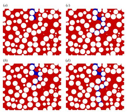
Figure 11. Time evolution of the liquid distribution on the YZ plane ( $X = 1.5 d_p$ ) at  $t/t^*$  of (a) 0.22, (b) 0.45, (c) 0.68 and (d) 0.91 displaying the trickle flow. Note: liquid and gas are coloured blue and red, respectively;  $AB_s = 1.85 \times 10^{-2}$ ,  $We_s = 5.92 \times 10^{-4}$ .
