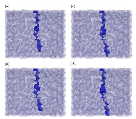
Figure 12. Dynamics of trickle flow with drop formation displayed using the liquid distribution at  $t/t^*$  of (a) 0.88, (b) 0.92, (c) 0.96, and (d) 1. Note: liquid is represented by iso-volume of  $\alpha_w \ge 0.5$  and is coloured blue, gas is transparent and particle surfaces are coloured grey;  $AB_s = 1.08 \times 10^{-2}$ ,  $We_s = 1.73 \times 10^{-3}$ .
