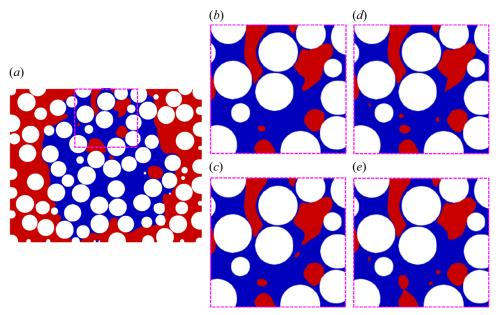
Figure 7. Liquid distribution on the YZ plane at  $X = 1.5 d_p$  at (a) breakthrough and enlarged view of the liquid distribution on the cut portion (marked by purple dashed lines) at  $t/t^*$  of (b) 0.567, (c) 0.574, (d) 0.581 and (e) 0.588 displaying the dynamics of inertia-induced bubble entrapment. Note: liquid and gas are coloured blue and red, respectively;  $AB_s = 2.37$ ,  $We_s = 3.79 \times 10^{-2}$ .
