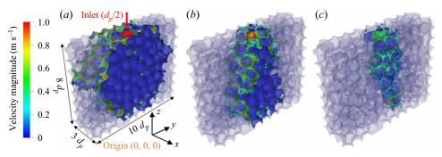
Figure 3. Liquid distribution (represented by iso-volume of  $\alpha_w \ge 0.5$  and indicated by blue colour) at  $AB_s$  of (a) 2.37, (b)  $2.01 \times 10^{-1}$  and (c)  $1.85 \times 10^{-2}$  at breakthrough ' $t^*$ ' (note: the two-phase interface (defined by iso-surface of  $\alpha_w = 0.5$ ) is coloured with the velocity magnitude. Further, the values of  $We_s$  and  $We_s$  and  $We_s$  are stated in table 1).
