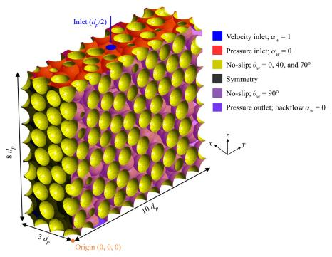
Figure 1. Computational domain with boundary conditions.
