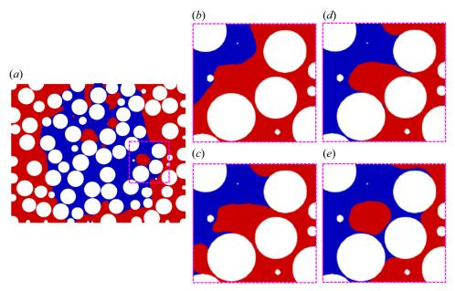
Figure 9. Liquid distribution on the YZ plane at  $X = 1.5 d_p$  at (a) breakthrough and enlarged view of the liquid distribution on the cut portion (marked by purple dashed lines) at  $t/t^*$  of (b) 0.67, (c) 0.73, (d) 0.79 and (e) 0.85 displaying the dynamics of capillary-induced bubble entrapment. Note: liquid and gas are coloured blue and red, respectively;  $AB_s = 2.37$ ,  $We_s = 3.79 \times 10^{-2}$ .
