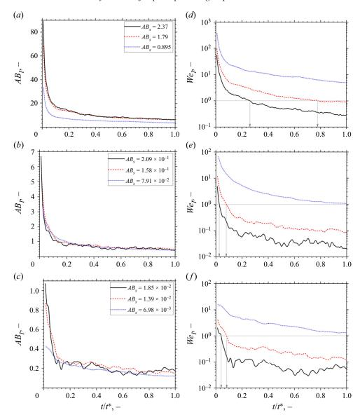
Figure 6. Time evolution of  $AB_I$  for liquid spreading influenced by (a) capillary or inertial force ( $AB_s \sim 1$ ), and that influenced (b) moderately ( $AB_s \sim 0.1$ ) and (c) strongly ( $AB_s \sim 0.01$ ) by gravitational force and  $We_I$  for liquid spreading influenced by (d) capillary or inertial force ( $AB_s \sim 1$ ), and that influenced (e) moderately ( $AB_s \sim 0.1$ ) and (f) strongly ( $AB_s \sim 0.01$ ) by gravitational force.
