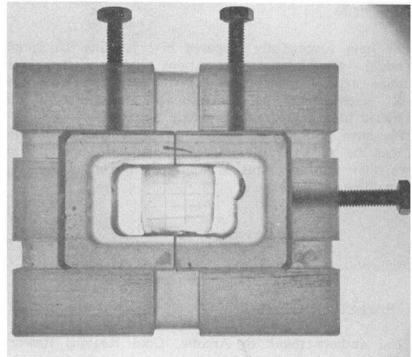
Fig. 2. Grip holder. The sample located in the central part of the apparatus has a rectangular section with a 15 mm fixed length. The width can range from 5 to 10 mm.
