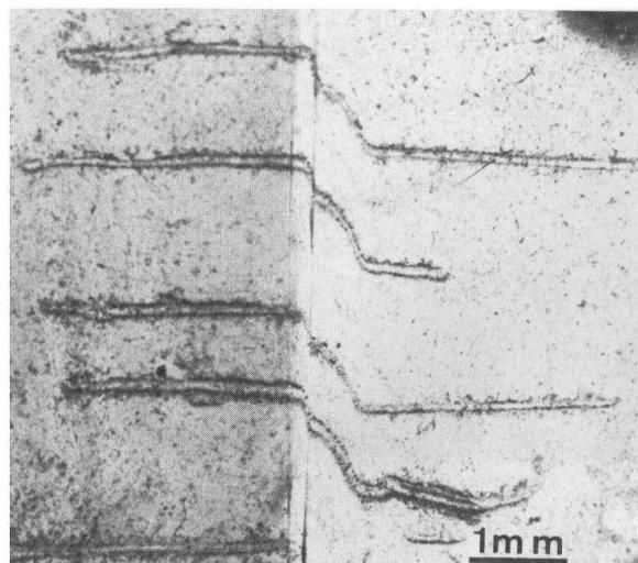
Fig. 3. Intense intragranular shear near a grain boundary.
