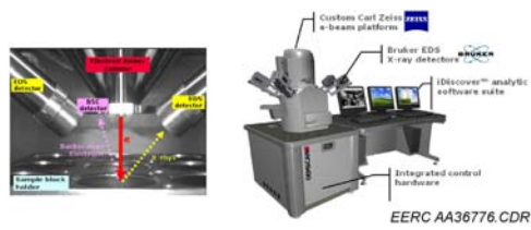
Figure 1. Main components of the QEMSCAN system.
