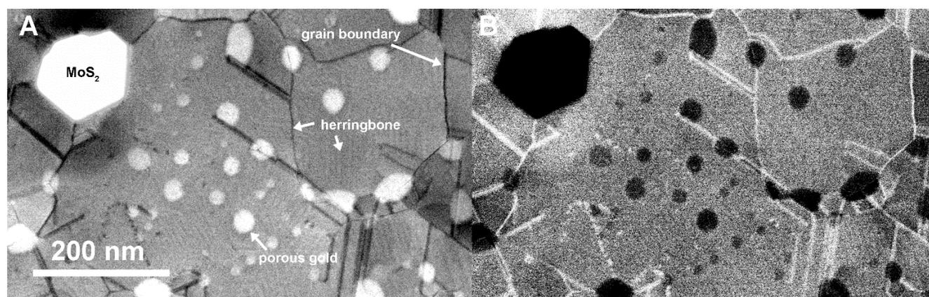
**Figure 2.** Low magnification STEM images of gold film with a monolayer MoS<sub>2</sub> 'pore'. (A) BF STEM shows thinner regions of gold appearing as bright circles and grain boundaries appear dark. A small intensity variation (labeled 'herringbone') strongly resembles the surface reconstruction of Au (111) seen with scanning tunneling microscopy. (B) HAADF STEM reveals inverted contrast from BF STEM for MoS<sub>2</sub> pore, grain boundaries, and thinner gold regions.
