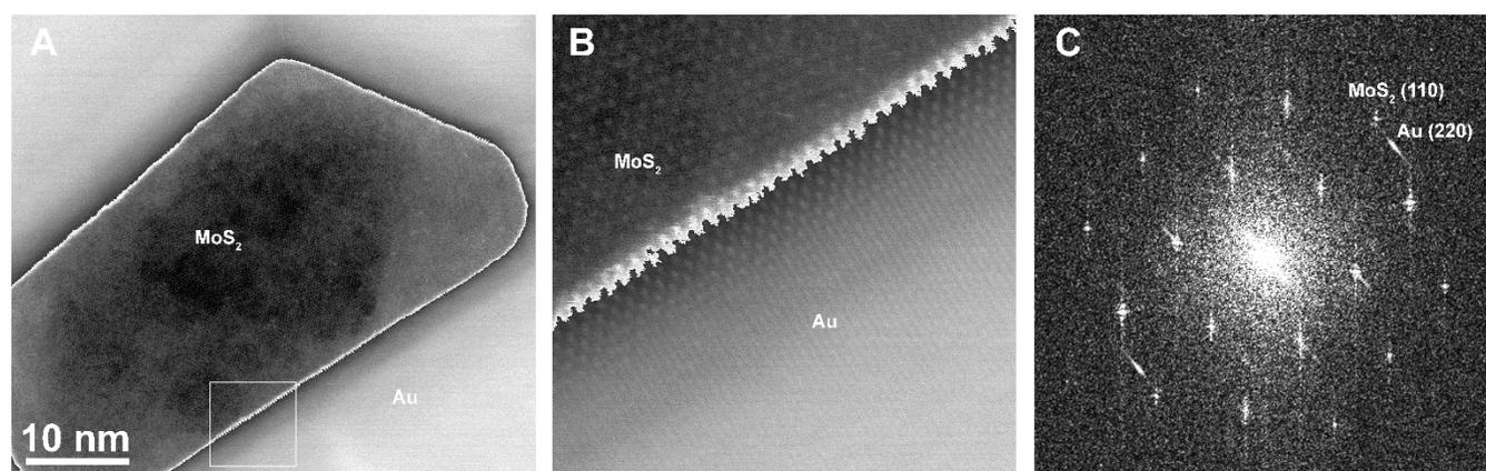
**Figure 1.** Aberration-corrected STEM of MoS<sub>2</sub> transferred onto gold thin films and annealed at 300°C. (A) HAADF micrograph of monolayer MoS<sub>2</sub> surrounded by a 25 nm thick gold film, with histogram equalization applied to each region separately. (B) A higher-magnification view of the indicated box in (A) showing the interface between MoS<sub>2</sub> and Au. (C) FFT of region shows registry of Au (220) and MoS<sub>2</sub> (110) lattice.
