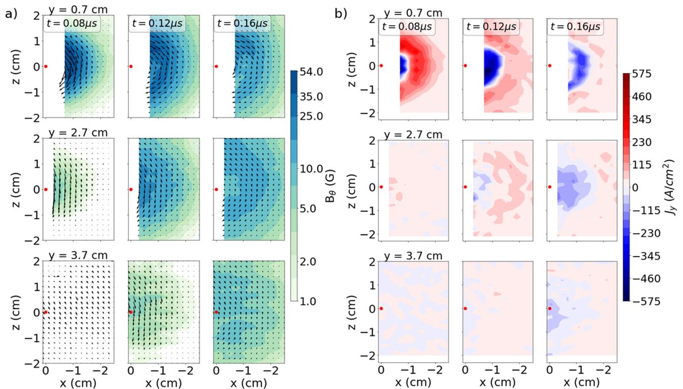
**Figure 2.** (a) Contour plots of azimuthal magnetic field structure in several transverse planes at three representative times. Magnetic field vectors are denoted by the black arrows. (b) The calculated current density along the plasma blow-off axis in several transverse planes at three representative times. The red dot represents the laser spot and white spaces are positions that the probe could not reach due to mechanical constraints.
