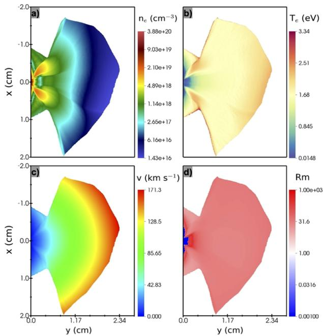
**Figure 7.** Visualization of the FBB 2D FLASH simulation for (a) the electron number density  $n_e$ , (b) the electron temperature  $T_e$ , (c) the magnitude of the velocity and (d) the magnetic Reynolds number at 150 ns after the laser fires. We describe the threshold applied to these visualizations in the text.
