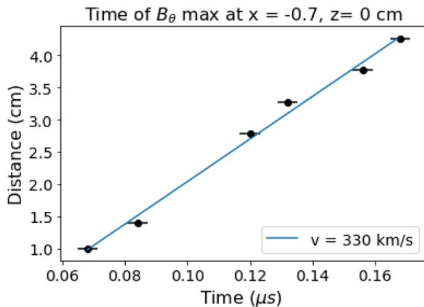
**Figure 5.** Plot of the maximum of the azimuthal magnetic field observed on the magnetic flux probe (black) at different planes as a function of time. A linear fit (blue line) to the data indicates a speed of  $330 \text{ km s}^{-1}$ .
