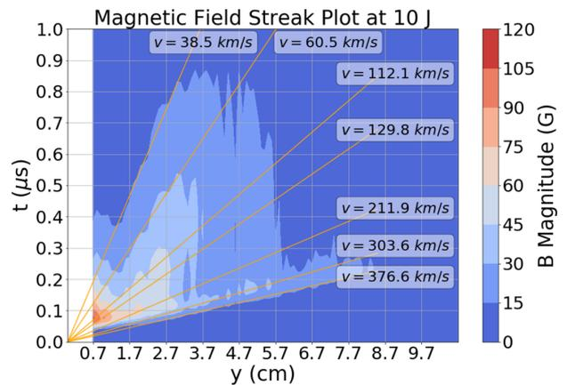
**Figure 4.** A streak plot of the total magnetic field (contour) from a  $y$ -lineout at  $x = -0.7$  mm,  $z = 0$  mm. Linear fits (orange lines) are applied to features of the magnetic field streak plot to determine the speed of different magnetic field features.
