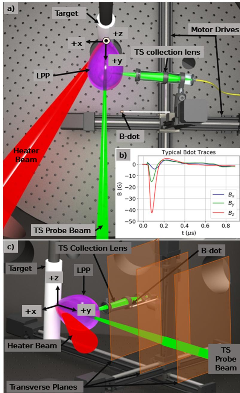
**Figure 1.** A rendering of the experimental setup. (a) Top view. The origin of the coordinate system is the laser spot on target, with the corresponding axis directions as depicted. (b) Typical B-dot probe traces for all three axes of the probe. (c) Side view. The translucent orange rectangles represent the planes in which magnetic field data were collected.
