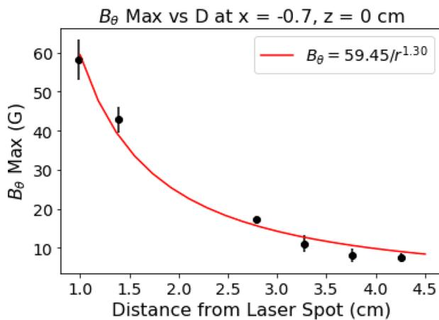
**Figure 3.** Plot of maximum azimuthal magnetic field versus distance from the laser spot. The times at which each point occurs correspond to the times in Figure 5. A  $1/r^a$  curve (red line) agrees well with the data with a value of  $a = 1.3$ .
