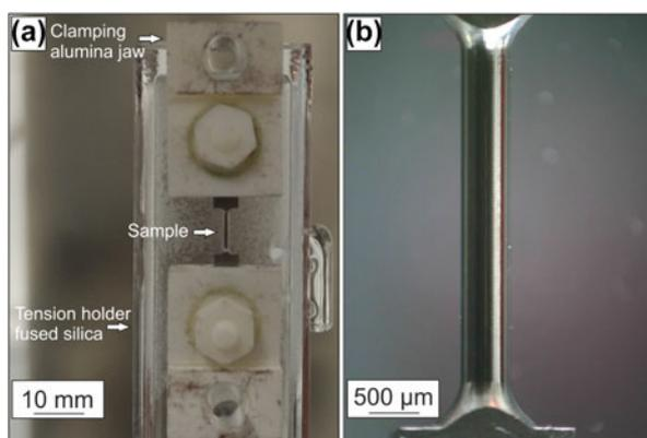
**Figure 8:** (a) TMA setup with fused silica tension holder, pushrod and clamping jaw made of alumina for mounting the (b) polished tensile specimen before creep testing with a diameter of  $450 \pm 2 \mu\text{m}$  over the entire gauge length of  $2500 \mu\text{m}$ .
