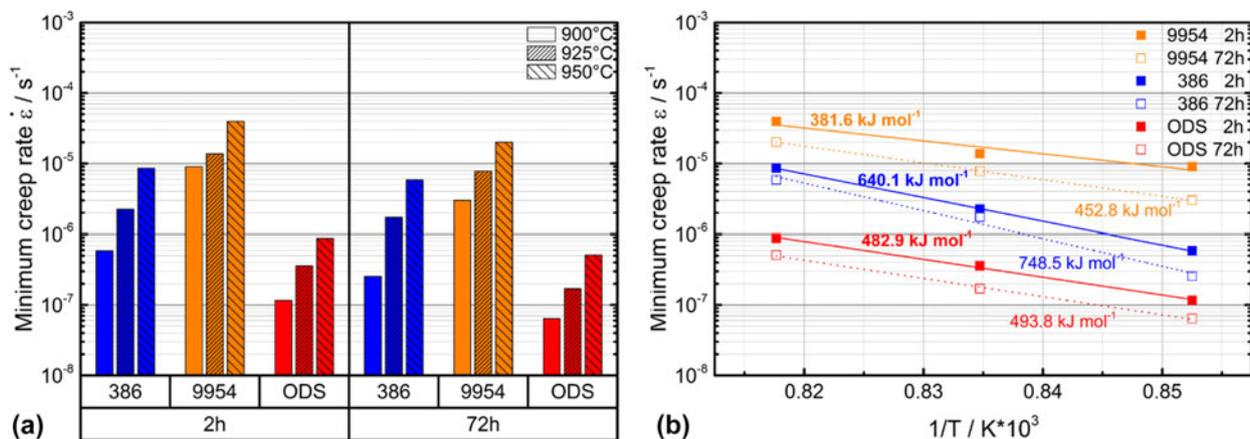
**Figure 4:** (a) Minima creep rates of Amdry 386, Amdry 9954 and Amdry 9954 + ODS at testing temperatures of 900–950 °C and an applied stress of 15 MPa after a first (2 h) and an additional second (72 h) heat treatment and (b) activation energies of all three bond coats at all testing temperatures.
