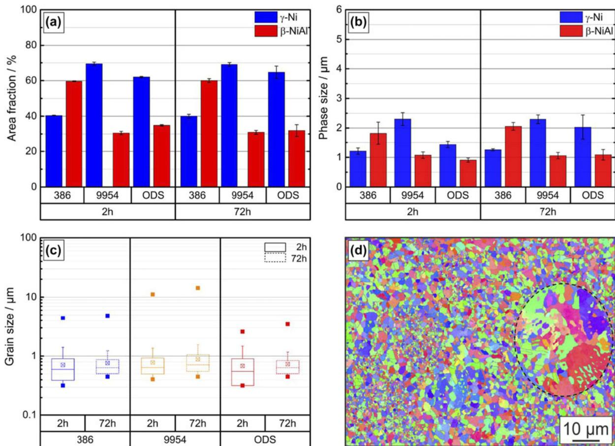
**Figure 2:** (a) Area fraction of phases and (b) phase size (c) grain sizes of Amdry 386, Amdry 9954 and Amdry 9954 + ODS after a heat treatment of 2 and 72 h at 1100 °C in vacuum before testing and (d) an EBSD mapping of Amdry 9954 with a large unmelted particle due to insufficient homogenization during thermal exposure.
