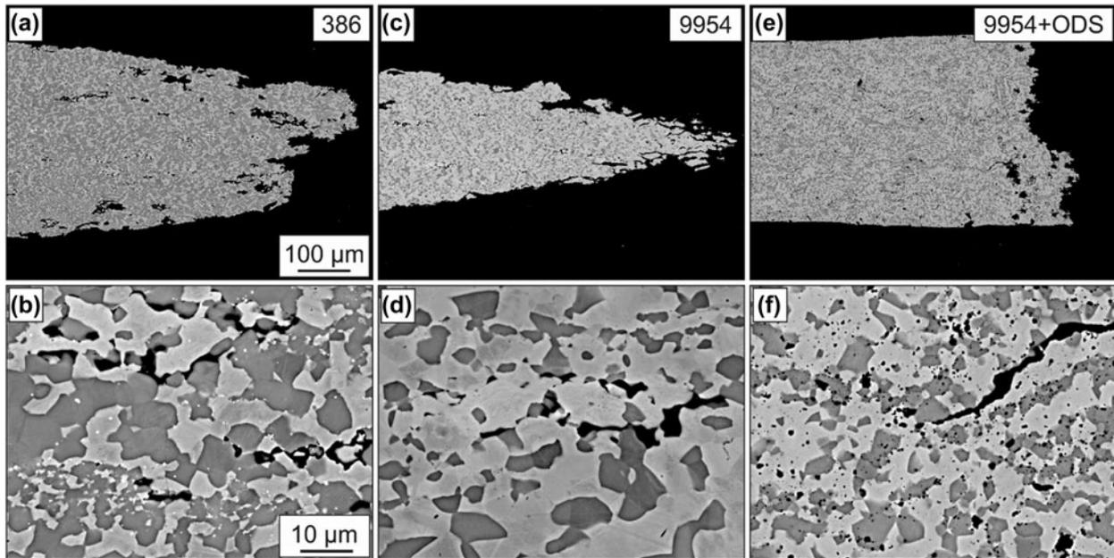
**Figure 5:** BSE images of the microstructures of Amdry 386 (a + b), 9954 (c + d) and 9954 + ODS (e + f) after 72 h of thermal exposure and microtensile creep tests at 950 °C.
