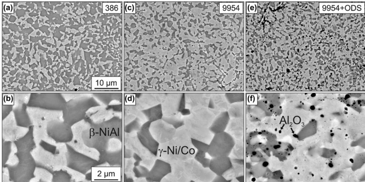
**Figure 1:** BSE images of the microstructures of Amdry 386 (a + b), Amdry 9954 (c + d) and Amdry 9954 + ODS (e + f) after a heat treatment of 2 h in vacuum at 1100 °C.
