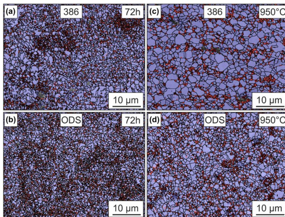
**Figure 7:** EBSD measurements after thermal exposure of 72 h of (a) Amdry 386 and (b) Amdry 9954 + ODS. EBSD measurements after the same heat treatment and microtensile tests at 950 °C for (c) Amdry 386 and (d) Amdry 9954 + ODS. Grains smaller than the median grain sizes (red) and grains larger than the medium grain size (purple).
