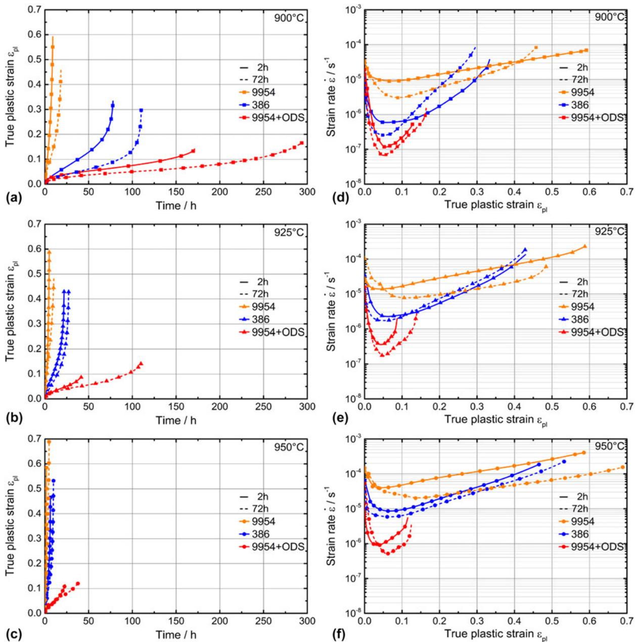
**Figure 3:** True plastic strain over time plot (a–c) and strain rate over true plastic strain plot (d–f) of Amdry 386, Amdry 9954 and Amdry 9954 + ODS after aging at 1100 °C for 2 h (solid lines) and 72 h (dashed lines) at testing temperatures of 900–950 °C with 15 MPa.
