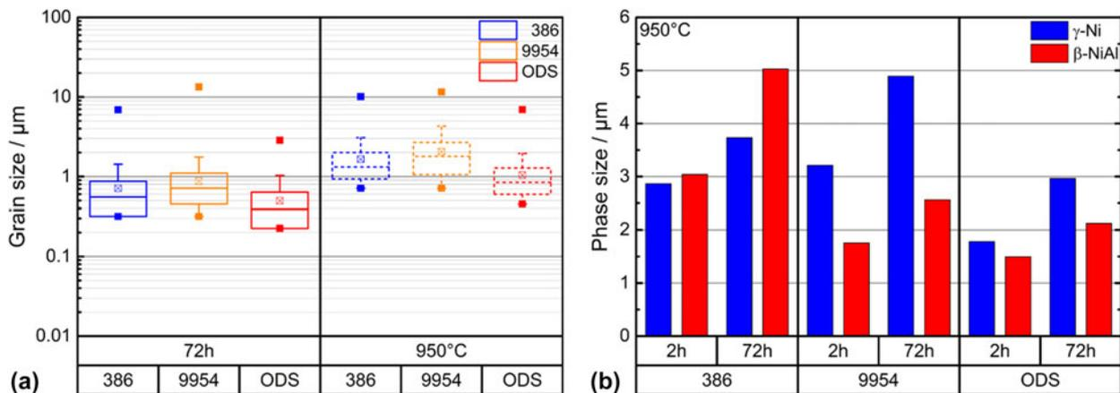
**Figure 6:** Grain sizes of Amdry 386, Amdry 9954 and Amdry 9954 + ODS (a) after 72 h of thermal exposure and after the same heat treatment and microtensile tests at 950 °C and (b) phase sizes after microtensile creep tests at 950 °C heat treated for 2 and 72 h at 1100 °C in vacuum.
