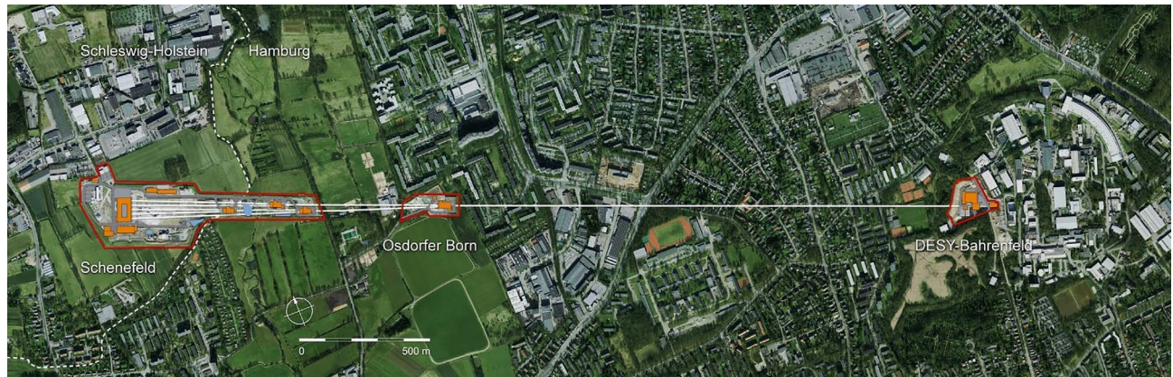
Figure 3. Layout of the European XFEL facility; the path of the underground tunnels is superimposed on a map of the northwest part of Hamburg and the town of Schenefeld in Schleswig–Holstein.
