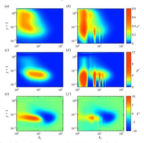
Figure 10. Contours of (a,b) spanwise spectra of turbulent kinetic energy  $e^+$ ; (c,d) spanwise spectra of production term  $p^+$ ; and (e,f) cumulative spanwise spectra of interscale transport term  $T^+$  at  $Re_{\tau}=180$  and  $Ro_{\tau}=5$ . (a,c,e) for R5J0 and (b,d,f) for R5J2B.
