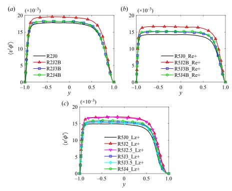
Figure 17. Convective scalar flux  $\langle v'\phi' \rangle$  in uncontrolled and controlled cases: (a)  $Re_{\tau}=180, Ro_{\tau}=2,$   $L_{z}=2\pi$ ; (b)  $Re_{\tau}=300, Ro_{\tau}=5, L_{z}=2\pi$ ; (c)  $Re_{\tau}=180, Ro_{\tau}=5, L_{z}=4\pi$ .
