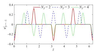
Figure 3. Spanwise distributions of wall-normal velocity in the injection/suction control at the bottom plate with different  $N_I$ .
