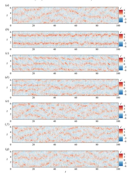
Figure 4. Contours of v'(0, 0, z, t) in the  $Ro_{\tau} = 5$  cases. The origin of t is chosen within a statistically steady state: (a) R5J0; (b) R5J2B; (c) R5J3B; (d) R5J4B; (e) R5J2T; (f) R5J3T; (g) R5J4T.
