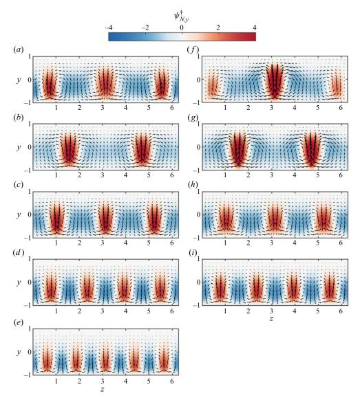
Figure 8. Velocity vectors in the *y*–*z* plane and contours of the wall-normal component of cluster centroids at  $Ro_{\tau} = 5$ : (a-e) R5J0, clusters  $C_1^{\dagger} - C_5^{\dagger}$ ; (f-i) R5J2B, clusters  $C_1^{\dagger} - C_4^{\dagger}$ .
