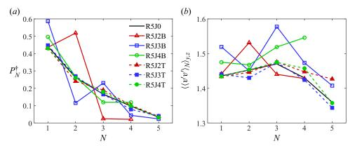
Figure 9. (a) Occurrence possibilities  $P_N^{\dagger}$  of clusters  $C_N^{\dagger}$  and (b) the y-z plane average of the conditional average of v'v' within clusters  $C_N^{\dagger}$  at  $Ro_{\tau} = 5$ .
