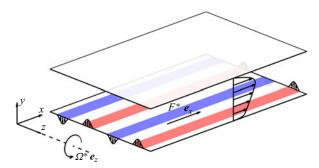
Figure 1. Sketch of the three-dimensional spanwise RPPF.
