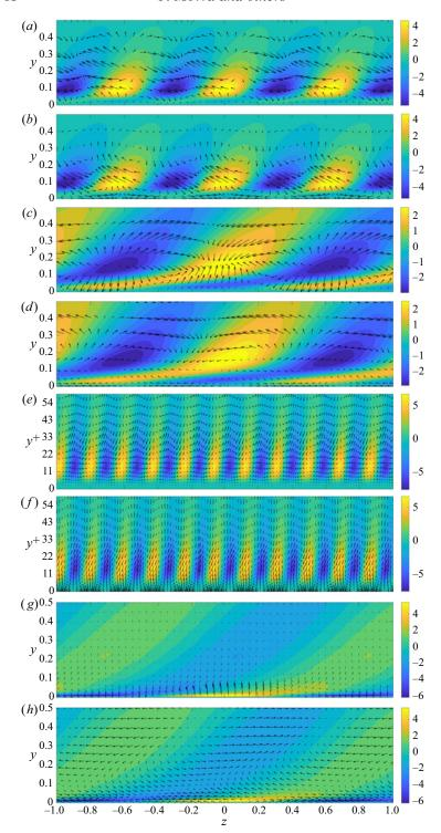
FIGURE 11. First SPOD mode of P,  $\zeta_1$ : (a-d)  $Re_{\tau} = 179$ ; (e-h)  $Re_{\tau} = 543$ ; (a,b,e,f) small scales; (c,d,g,h) large scale; (a,c,e,g) full  $\zeta_1$ ; (b,d,f,h) solenoidal part of  $\zeta_1$ . Contours: streamwise component of  $\zeta_1$ . Vectors: spanwise and wall-normal components of  $\zeta_1$ .
