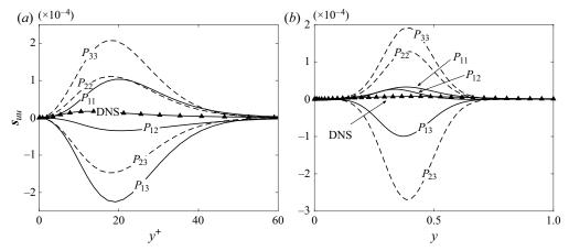
FIGURE 8. Response  $\mathbf{S} = \mathbf{R} \mathbf{P}_{ij} \mathbf{R}^H$  from sub-blocks of  $\mathbf{P}_{ij}$ , with  $Re_{\tau} = 179$ : solid lines, response from  $\mathbf{P}_{1j}$  (sub-blocks related to the streamwise component); dashed lines, response from  $\mathbf{P}_{ij}$  with  $i \neq 1$ ; (a)  $s_{uu}$  near-wall,  $\omega_{max}^+ = 0.065$ ; (b)  $s_{uu}$  large scale,  $\omega_{max} = 1.05$ .
