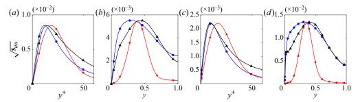
FIGURE 14. PSD. Streamwise component  $s_{uu}$ : (a,b)  $Re_{\tau}=179$ ; (c,d)  $Re_{\tau}=543$ ; (a,c) small scale; (b,d) large scales. Black line with triangles: DNS data. Red line with squares:  $\mathbf{S}_{\nu}=\gamma_{\nu}\mathbf{R}\mathbf{R}^{H}$ . Blue line with circles:  $\mathbf{S}_{\nu_{\tau}}=\gamma_{\nu_{\tau}}\mathbf{R}_{\nu_{\tau}}\mathbf{R}^{H}_{\nu_{\tau}}$ .
