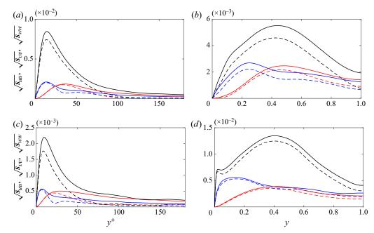
FIGURE 10. PSD of the velocity fluctuations from the low-rank approximation: solid lines, **S** from DNS data; dashed lines,  $\mathbf{S}_{lr}$  from low-rank approximation of  $\mathbf{P}_{lr}$ ; black, streamwise component; red, wall-normal component; blue, spanwise component; (a)  $Re_{\tau} = 179$ , small scale; (b)  $Re_{\tau} = 179$ , large scale; (c)  $Re_{\tau} = 543$ , small scale; (d)  $Re_{\tau} = 543$ ; large scale.
