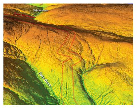
FIG. 26. Oblique LiDAR view showing the descent into the Hindburn valley and the previously unknown large dog-leg. (© *D. Ratledge. Base LiDAR data* © *Crown Copyright*)
