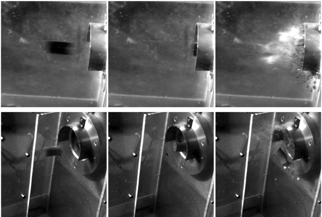
FIG. 2. High speed video frame sequence of two valid impact tests: glass specimen at impact speed of  $60 \text{ m s}^{-1}$  (top images); grit in grout specimen at impact speed of  $28 \text{ m s}^{-1}$  (bottom images).
