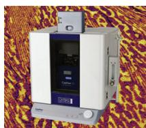
Oxford Instruments/Asylum Research has announced their new Cypher VRS1250 video-rate atomic force microscope (AFM) with scan rates up to 1250 lines/second and frame rates up to 45 frames/second. This speed enables capture of nanoscale details of dynamic events, including biochemical reactions, 2D molecular self-assembly, and etch and dissolution processes. The system supports a range of modes and accessories, making it a versatile tool for interdisciplinary research groups.
