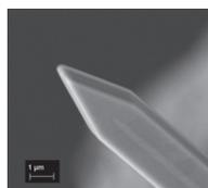
ICSPi has announced two additions to the nGauge AFM product line-up. New sharp, diamond-like carbon tips offer the best lateral resolution and highest fidelity imaging on the nGauge AFM, enabling new applications. New AFM wedge tips offer a unique sharpened "wedge" design for robustness and consistency and are ideal for general-purpose imaging and pre-screening samples.
