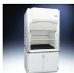
The HEMCO Auxiliary Air fume hood exhaust requires no room air. With the sash in the half-open position and face velocity of 100 feet per minute, the cfm required equals the hood air supply. Exhaust plus auxiliary air make up for room supply deficiencies. When there is a shortage of air in the lab, it is less costly to provide an Auxiliary Air fume hood system than to change or enlarge the whole building air handling system.
