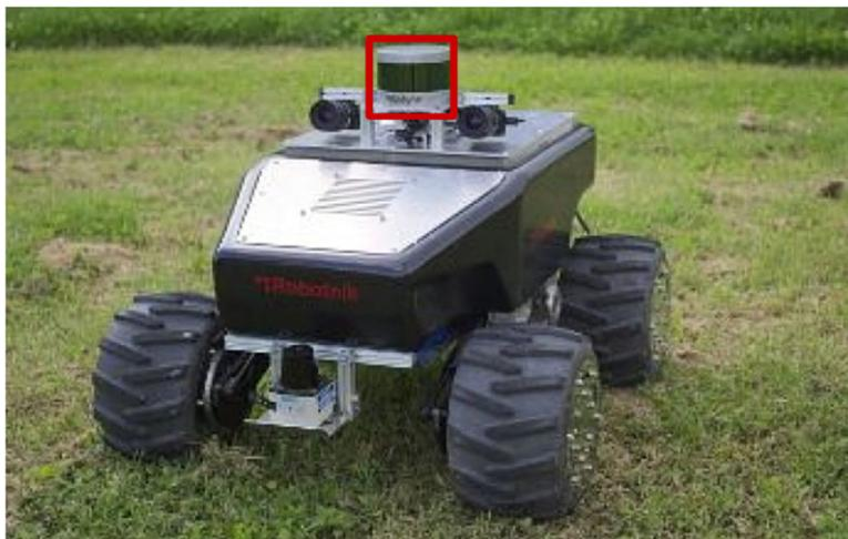
**Figure 10.** Experimental setup for lidar data acquisition. The lidar sensor is highlighted in red on the picture. The lidar sensor operates with a 360° vertical field of view ( $\sim 0.2^\circ$  angular resolution) and a  $\pm 15^\circ$  vertical field of view ( $2.0^\circ$  angular resolution).
