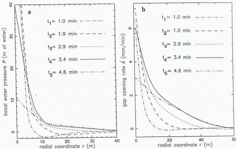
Fig. 22. Empirical calculation of gap-growth rate based on observation of water-pressure distribution  $P(r, t)$  in the pressure-pulse propagation experiment. (a) Empirical curves of  $P(r, t_i)$  at selected times  $t_i$  as indicated, based on observations and assumptions noted in the text (section 9c). (b) Corresponding gap uplift rates  $\delta(r, t_i)$ , based on Equation (17). These are used to calculate by integration the volume of water stored at the different times (see text).
