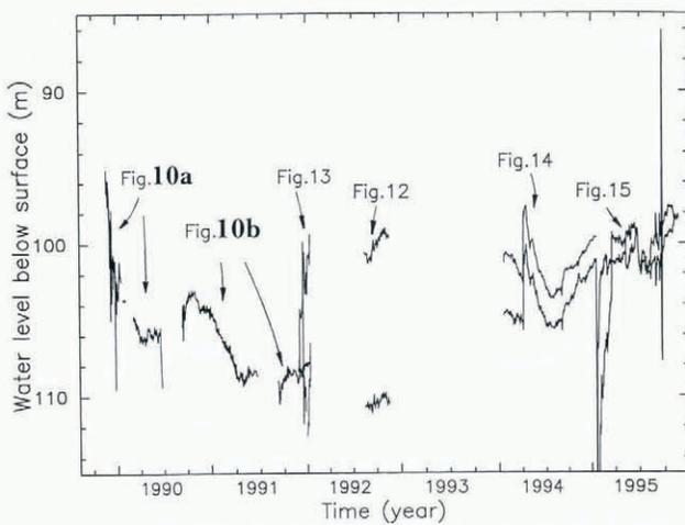
Fig. 8. Measured basal water pressures over the 6 year period 1990–95. The arrows refer to the figures that give expanded plots of parts of the complete record as indicated and that identify which boreholes are the sources of the various traces shown.
