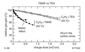
Fig. 12.3. Comparison of wire-chamber ageing in multiwire proportional chambers filled with  $C_2H_6$ +TEA versus  $C_2H_6$ +TMAE for a fixed anode-wire diameter in its dependence on the deposited charge on the anode wire [16].
