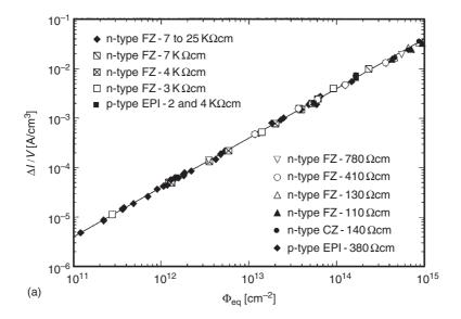
Fig. 12.6. Reverse current of different silicon detectors produced by various technologies induced by the exposition to an equivalent fluence  $\Phi_{eq}$ . The measurements were performed after a heat treatment for 80 min at 60 °C [28].
