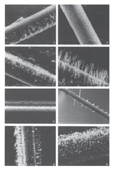
Fig. 12.4. Examples of depositions on anode wires [3].
