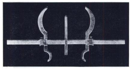
The Instrument is well finished in brass, nickel-plated. The graduated bar is of German silver.
