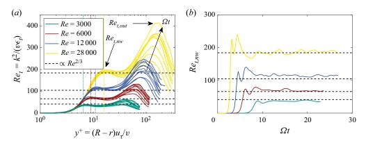
Figure 9. The DNS data of Kaiser *et al.* (2020): (a) turbulent Reynolds number  $Re_t$  during stage III with a time-invariant near-wall plateau, which is described through its peak value  $Re_{t,nw}$  at a time-invariant wall-normal location (vertical dotted lines); and (b) temporal evolution of  $Re_{t,nw}$  during stages I–III. The dashed horizontal lines indicate proportionality to  $Re^{2/3}$ .
