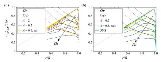
Figure 7. Influence of (A) and the presence of a salt-water layer on the flow characteristics during spin-down experiments. Five time instances  $\Omega t \in \{2, 8, 16, 32, 64\}$  are presented. The SBR and regions of constant angular momentum l(t) are emphasised using dotted and dashed lines, respectively. (a)  $Re = 5.6 \times 10^4$  and (b) comparison of experimental results with DNS data from Kaiser et~al.~(2020) at  $Re = 2.8 \times 10^4$ .
