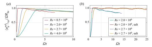
Figure 8. End-wall effects and their reduction. While  $\langle u_{\varphi}^{rel} \rangle_{r,\varphi}/\Omega R_{hs} \approx 1$ , the core is still in SBR. The ramp of of the acceleration/deceleration process varies for different Re. The experiments where a saturated salt-water layer was introduced are marked with the tag 'salt'.
