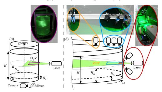
Figure 2. Set-up of the SSE (a) and the LSE (b). Stereo PIV system focused on the near-wall region (red), planar PIV system covering the long-term boundary-layer evolution (blue), and planar PIV to assess the coherence of the vortex core (orange). Filling height H, axial position of the measurement plane  $H_m$  and height of the saturated salt-water layer  $H_s$ .
