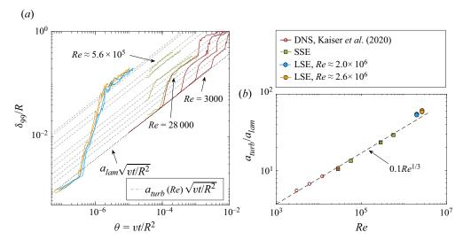
Figure 5. (a) Boundary-layer growth  $\delta_{99}$  at various Re. The plotted curves correspond to  $Re \in \{0.3, 0.6, 1.2, 2.8\} \times 10^4$  (DNS, Kaiser et al. 2020),  $Re \in \{2.8, 5.6\} \times 10^4$  (SSE, salt, A = 0.5),  $Re \in \{2.8, 5.6\} \times 10^5$  (SSE, no salt, A = 2.0), and  $Re \in \{2.0, 2.7\} \times 10^6$  (LSE, salt, A = 2/13). Dashed lines show the suggested empirical Re scaling of turbulent boundary layers (3.2); and (b) Re scaling of  $a_{Iurb}/a_{lam}$ .
