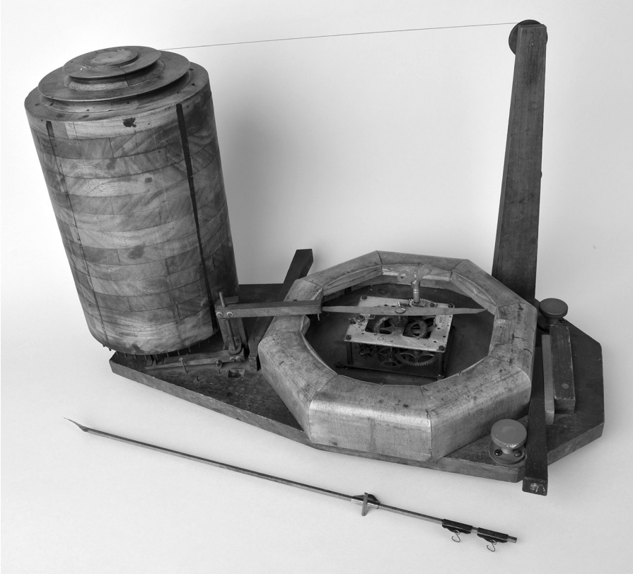
Auxanometer built by Horace Darwin in 1876. © Whipple Museum (Wh.2766).
