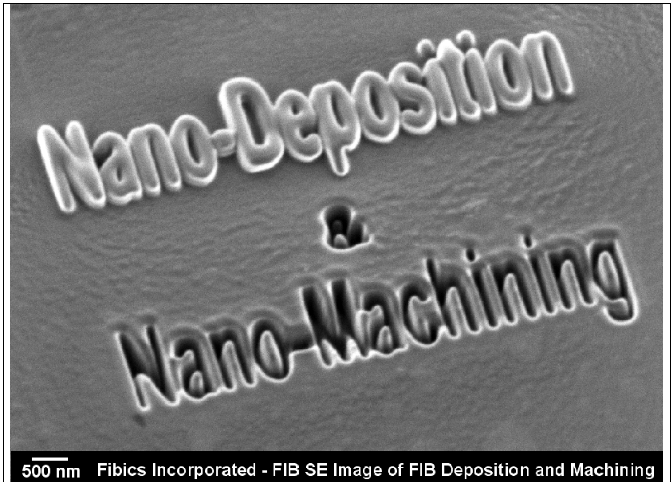
FIG. 1. FIB deposition can produce features 200 nm or less in thickness. FIB milling can produce even finer results. This structure required approximately 30 minutes of FIB time to produce.
