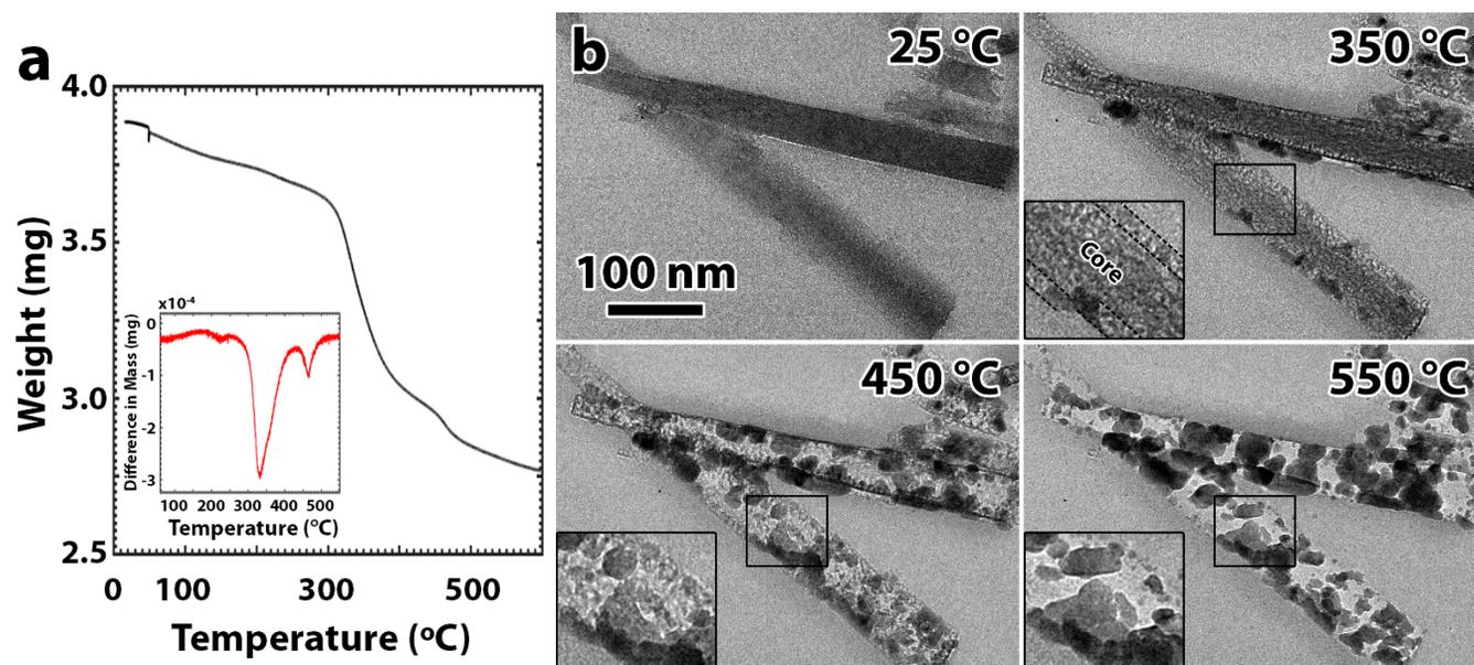
**Figure 1.** (a) TPR analysis of the NiMoO<sub>4</sub> nanorod reduction. The inset shows the first derivative of the data, to more clearly visualize the inflection points, (b) Micrographs from the *in situ* TEM reduction in H<sub>2</sub> showing the corresponding structures formed at the key transformation temperatures. The dashed lines in the inset bound the Ni-depleted layers.
