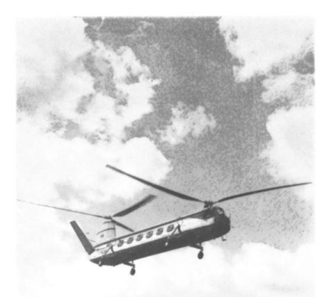
The Bristol 173 Helicopter is fitted with two Alvis Leonides Engines
