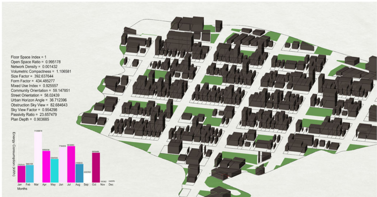
Fig. 19. A picture screen of the output of the software. The urban setting that was created by the tool is shown on the right, its values of urban form are shown on the top left, and the predicted values of energy consumption are shown on the bottom left.
