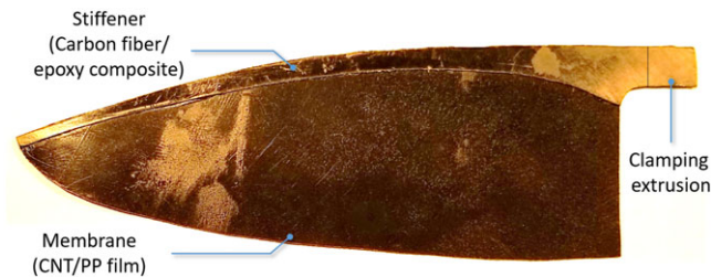
Figure 6. The fabricated model of the hummingbird-inspired wing (HIW).
