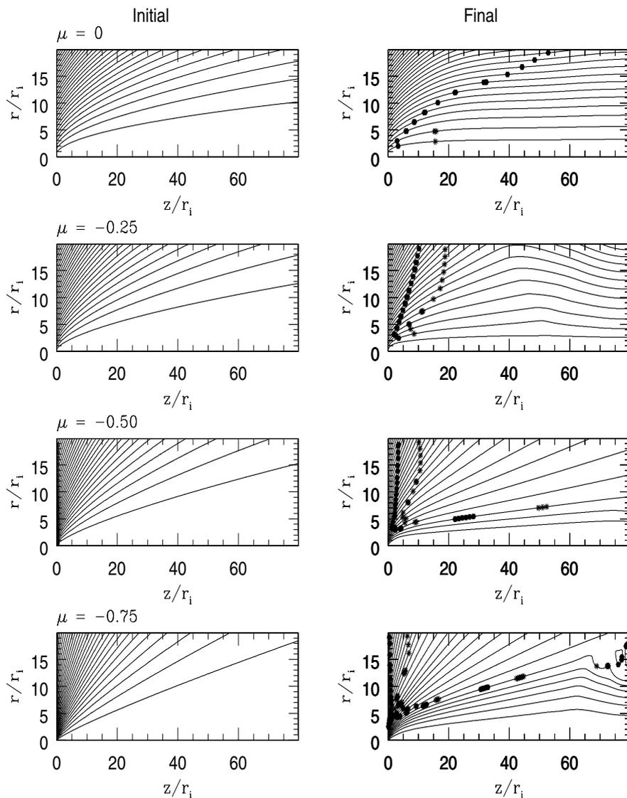
**Figure 1.** Initial (left panels) and final (right panels) magnetic configurations for disk winds for 4 models of the disc magnetic field. From top to bottom these are the potential solution, BP, PP, and a steeper  $\mu = -0.75$  configuration (see equation 3.12). Outflows are less well collimated as one goes from top to bottom. (Adapted from PRO05).
