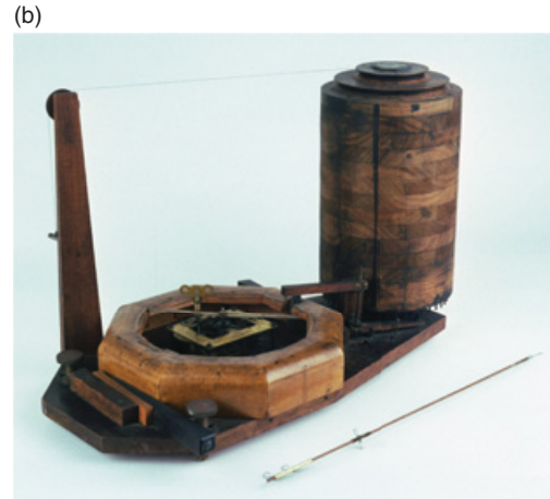
Figure 7.2b Horace Darwin's self-recording auxanometer
