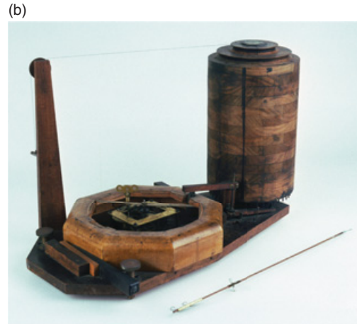
Figure 7.2b Horace Darwin's self-recording auxanometer
